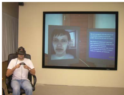
Figure 2. View of the HMD and the projection screen.
